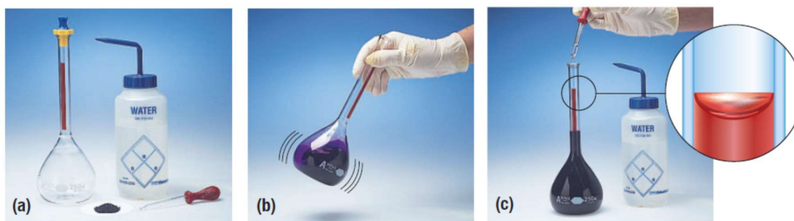
Figure 5 (a) To prepare a 250 mL sample of potassium permanganate solution, you will need a volumetric flask, distilled water, a dropper, and the required mass of potassium permanganate, \text{KMnO}_4 . (b) First dissolve the solid \text{KMnO}_4 in about 100 mL of distilled water. (c) Use a dropper to add distilled water until the bottom of the meniscus lines up with the calibration mark on the flask.
